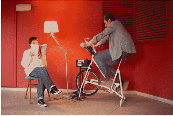
Image: The friction drive – a small roller attached to the generator shaft and pressed against the flywheel.
