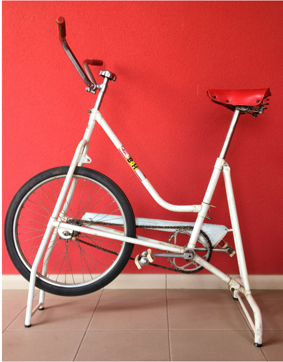
Image: The exercise bike dating from the 1950s. It has a heavy flywheel in front.
